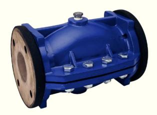
Rhinoflex Series-PJ, Air Jacketed pinch valves offers a simple, cost-effective design, perfect for handling extremely demanding abrasive materials. The valve's split body design allows quick and easy sleeve replacement, and is available in ductile iron, with flanged ends.
